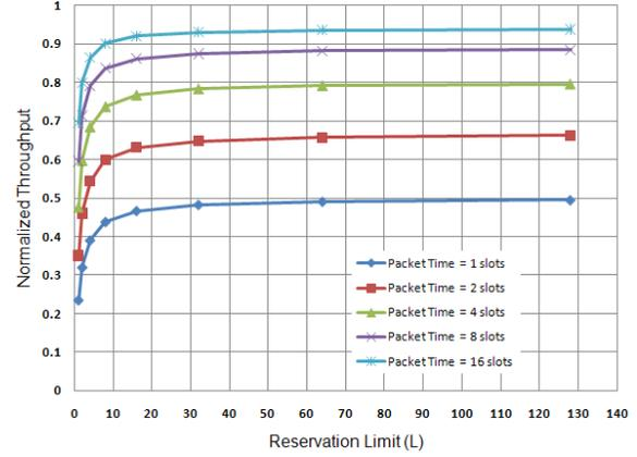
Fig. 4. Normalized throughput versus Reservation Limit for packets of different sizes. The number of nodes is 25 and optimal contention window is assumed.
