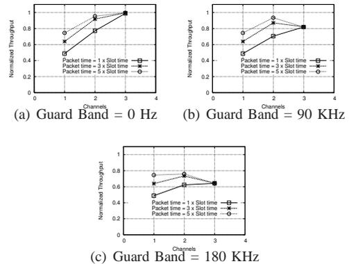
Fig. 8. Throughput vs. number of channels and packet size for different guard bands.
