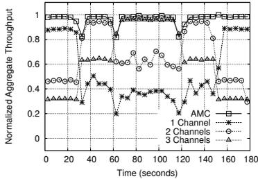
Fig. 9. Benefits of adaptive channelization compared to fixed channelization. (Packet time = 1 slot time. Zero guard band.)
