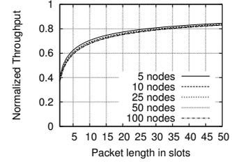
Fig. 1. Normalized throughput versus packet time (in slots) for a single channel 802.11-like network. Optimal contention window is assumed.
