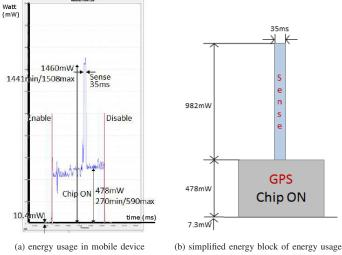
Fig. 7. Energy usage of the GPS chip in a mobile device.
