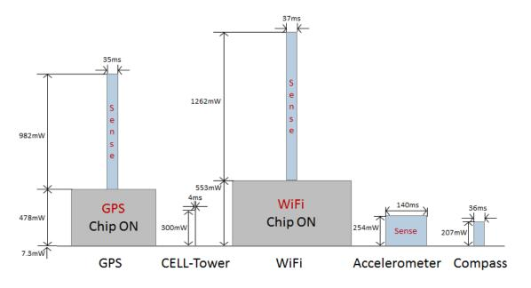
Fig. 8. Energy usage profiles for GPS, 3G, WiFi, accelerometer and compass.
